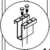
Attach grating to Hat Channel using MHC25 Hold Down Clamp and (2) 12-14x<sup>3</sup>/<sub>4</sub>" Fasteners. CAUTION: Be sure fastener does not penetrate ribs.
