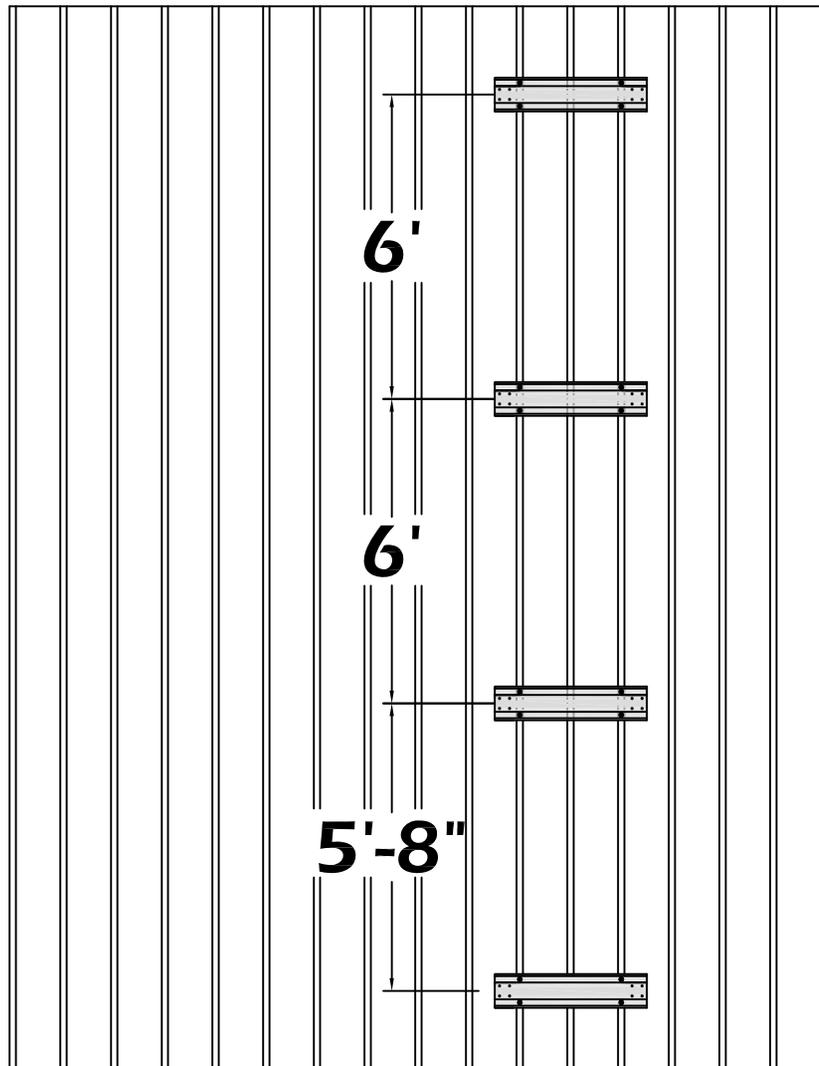
1- Using roof layout diagram, locate Support plates for parallel runs. Use same procedure for Handrail and Non-Handrail jobs. Rest Support Plates on roof panel. Field drill (4)  $\frac{5}{16}$ " holes thru Support Plate and panel high ribs.
