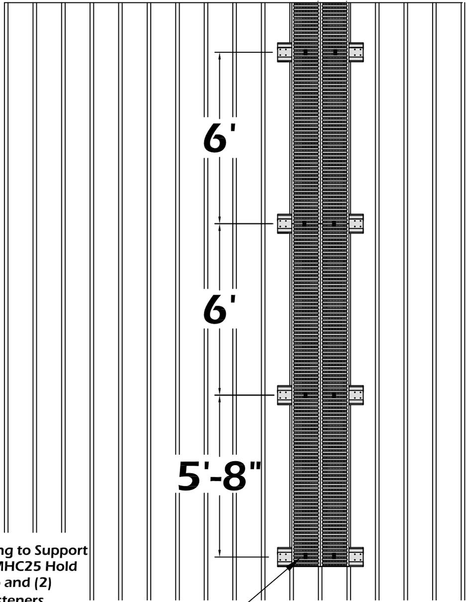
Attach grating to Support Plate using MHC25 Hold Down Clamp and (2) 12-14x<sup>3</sup>/<sub>4</sub>" Fasteners.
