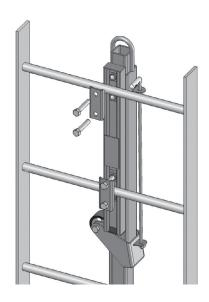
LadderUP Safety Posts provide easier, safer ladder access through roof hatches, floor access doors and manholes. This telescoping post permanently mounts to the top two rungs of any fixed ladder, providing a positive hand-hold and enabling the user to enter or exit an opening in an upright and balanced position.
