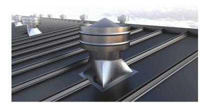
The Moffitt SG (Stationary Gravity) ventilator is a round, non-moving vent that is used to exhaust warm air. It is used on many industrial and commercial applications. They are designed to withstand winds up to 85 miles per hour and are waterproof and storm proof under all normal operating conditions. Each unit is designed to stay free from back drafts in ideal conditions.
